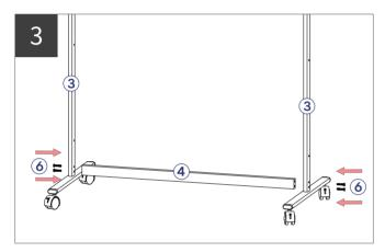
Connect the crossbar (4) on the installed columns (3) by M4\*35mm screws (6)
