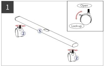
Install the castor wheels (2) on the foot bar (5)
