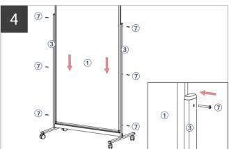
Install the whiteboard (1) between the two columns(3) from top to bottom by M4\*30mm screws (7)
