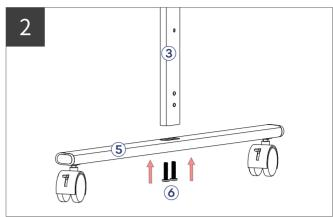
Install the foot bar (5) on the column(3) by M6\*35mm screws (6)
